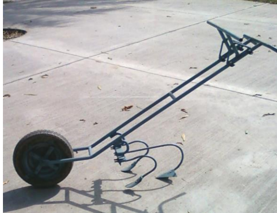
Fig. 14. Manually operated multipurpose toolbar with single row three tined intercultivator attachment
