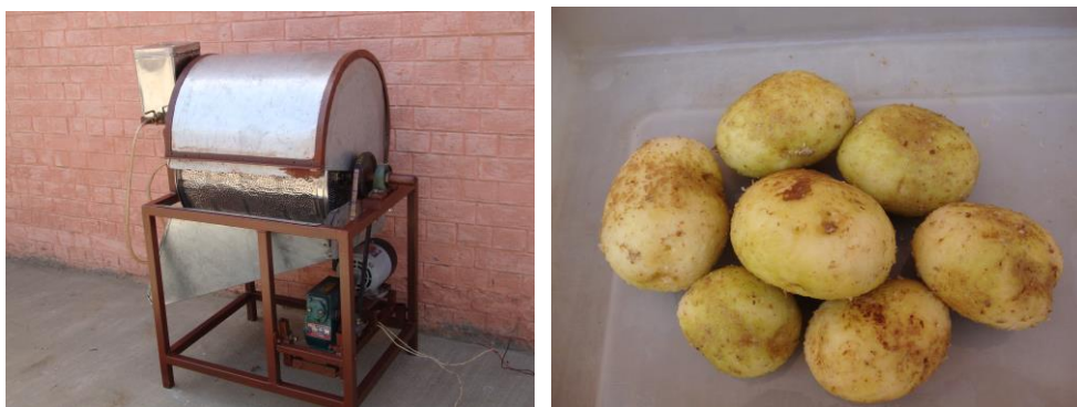
Fig. 15. Power operated potato peeler and a view of potato peeled with prototype peeler
