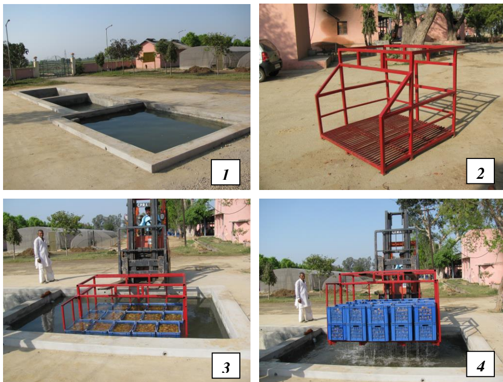
Fig 18. (1) Washing/treatment channels, (2) perforated pallet, (3) dipping of tubers for washing and (4) washed tubers ready for treatment
